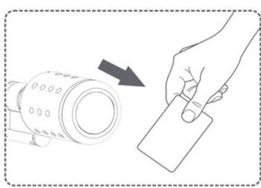
3 An acoustic signal is sounded and the LEDs blink red and blue three times. The coupler is actuated.
