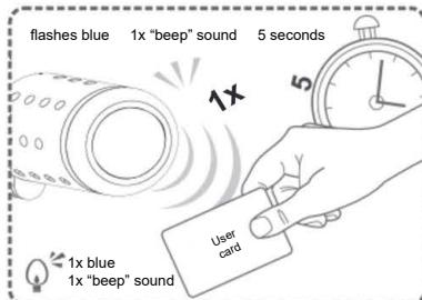
2 To deactivate the passage mode, the user medium must be held in front of the cylinder for 5 seconds or the open button in the app must be pressed for 5 seconds.
