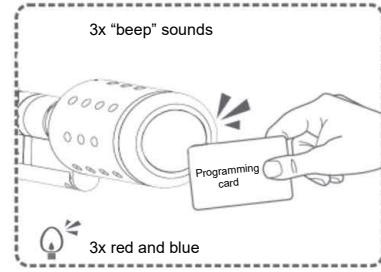
5 If the programming card is removed within the aforementioned 10 seconds, the "learning process" fails.
